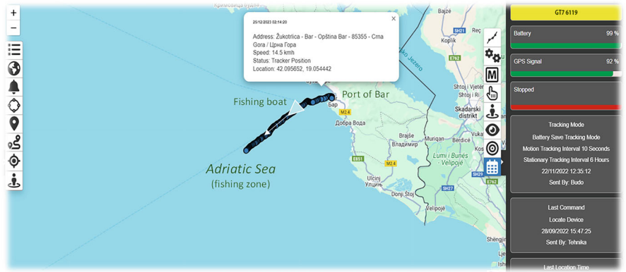
Fig. 7 Web application for tracking the container at sea: A dispatcher’s view (own research)
