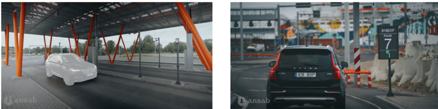
Fig. 3 Taking snapshots of the vehicle and reading its key physical parameters (a); digital displays for guiding the vehicles to the right gathering zone and waiting line (b) [16]
